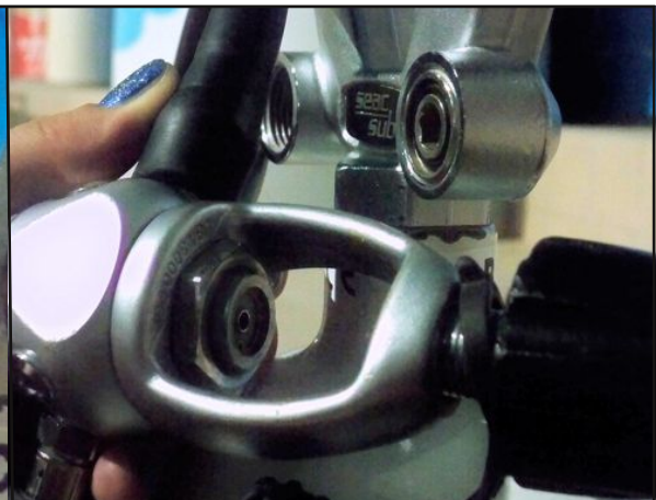
Yoke fitting - valve with O ring
